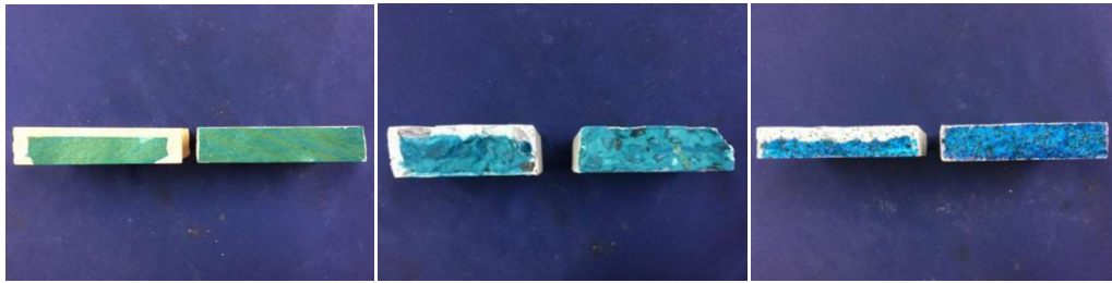
Fig. 1. Penetration depth test: sandstone (left), wet-cast concrete (middle) and granite (right).
